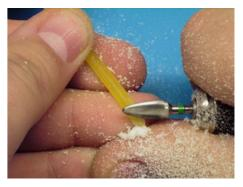
Hardened patterns can be adjusted by grinding or milling.
